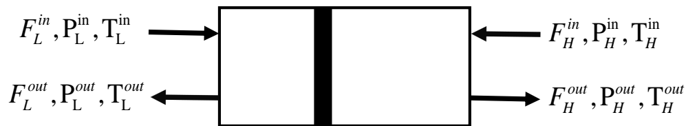
Figure 5.2. Schematic representation of a work exchanger module.
